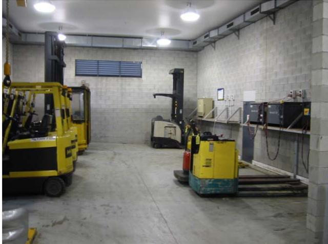
There have been a number of reported fire losses involving these units, principally during the recharging process. Insulation, battery boxes and accumulated grease deposits on battery powered trucks are combustible material which may become ignited and involve the truck in fire.
